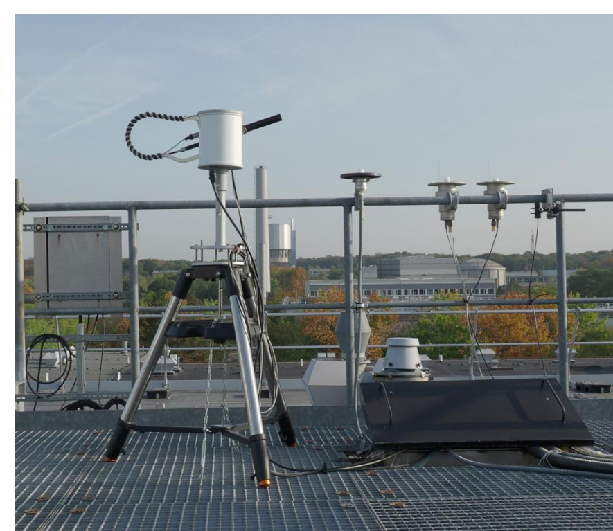
Pandora system and Avantes zenith-sky system installed in Jülich, next to routinely operated instruments
